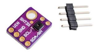
If you're using an Arduino simply connect the VIN pin to the 5V voltage pin, GND to ground, SCL to I2C Clock (Analog 5) and SDA to I2C Data (Analog 4).
